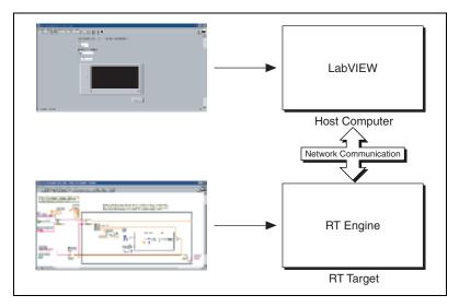
Figure 1-1. Front Panel Communication Protocol
