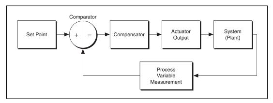
Figure 5-1. Typical Control System
