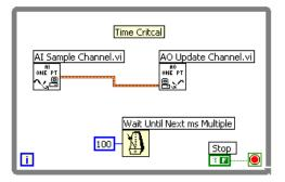
Figure 5-4. Parallel Implementation of a Control System
