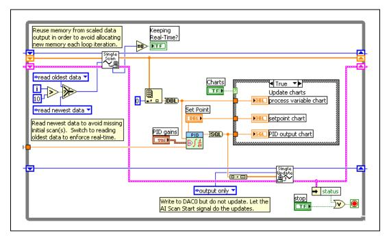
Figure 5-13. One Channel PID Output
