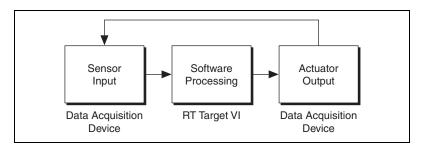
**Figure 5-2.** Typical LabVIEW Control Application
