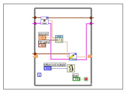
Figure 5-14. One Channel PID Output Using FieldPoint
