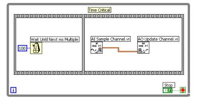
**Figure 5-6.** Flat Sequence Implementation of a Control System
