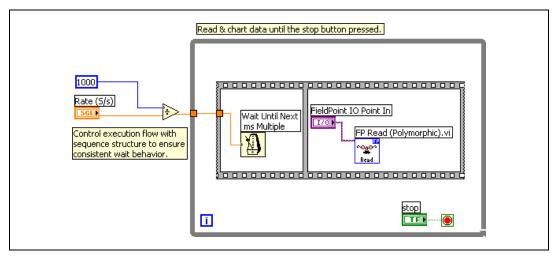
Figure 5-10. Acquiring Data Using FieldPoint
