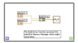
Figure 6-1. Memory Allocation in Control Loop
